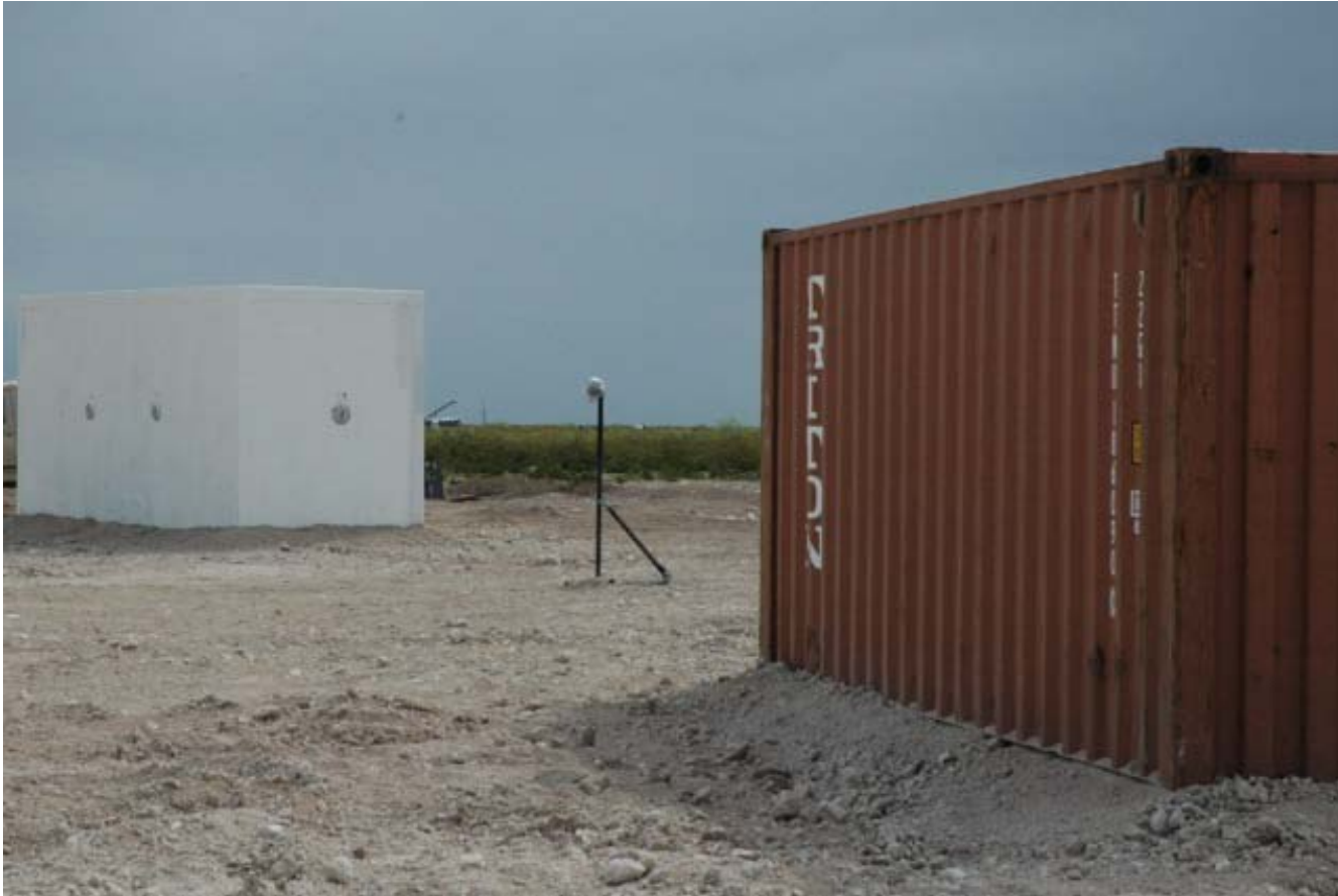
BRM 3, incident transducer radial, and connex container as deployed
